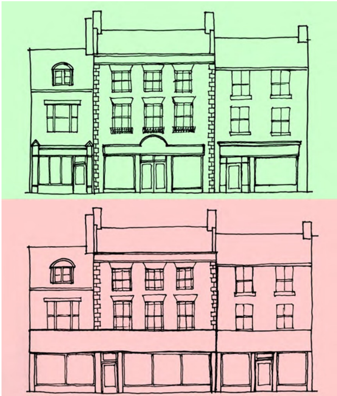
Figure 23 - The specific character of each building is reflected in the design of shopfronts in the top image, but ignored when the ground floors are amalgamated into one large unit.
